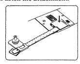
\* Match the attachment to left side of the attachment holder hole and press it down where the arrow shows.
