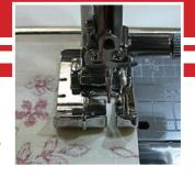
The 1/4" Seam Foot with no guide plate attached is a very useful tool for various types of piecing work. As with the 1/4" seam foot, you can sew the 1/4" position by aligning the cloth with the edge of the presser foot. While the
