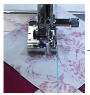
Align the edge of foot with the mark and sew.
