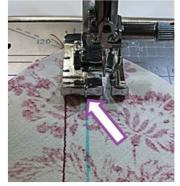
Match the 1/4" guide line with the mark and sew. As the guide line is raised, it is easy to align with the mark.
