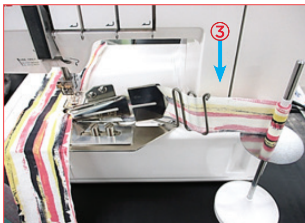
Supply the tape at the same height as the binder
