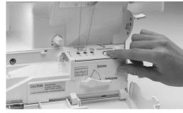
RevolutionAir™ Looper Threading Insert thread into one of the Triumph's threading ports, push the button and a gust of air quickly pushes it through the patented tubular loopers, exactly where you need it every time.
